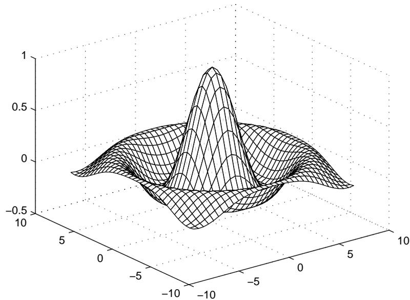
By default, MATLAB colors the mesh using the current colormap. However, this example uses a single-colored mesh by specifying the `EdgeColor` surface property. See the surface reference page for a list of all surface properties.
