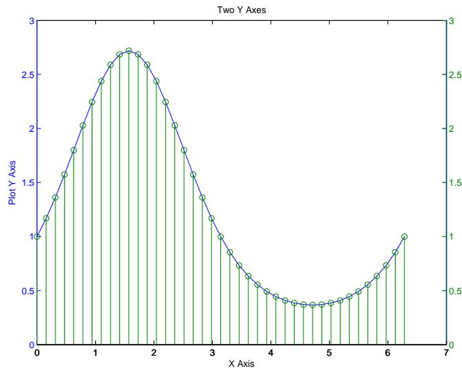
This graph contains two *y*-axes, one for each plot type (lineseries and stem graphs). The plotting tools make it easy to select any of the objects that the graph contains and set their properties.
