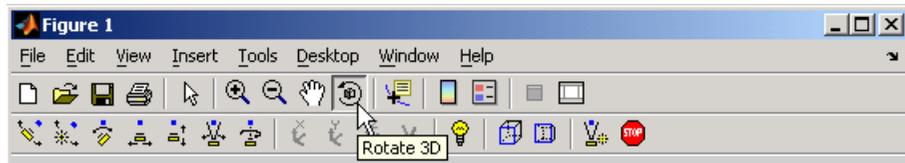
These tools enables you to move the camera around the surface object, zoom, add lighting, and perform other viewing operations without issuing commands.
