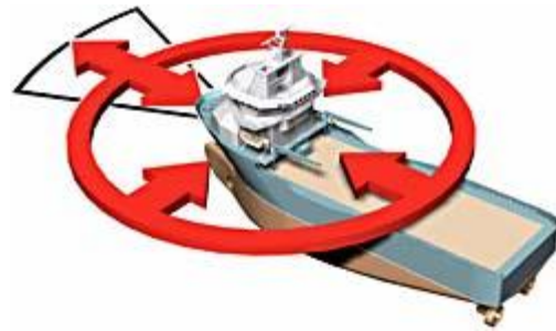
Dynamic positioning system - illustrating auto position mode
